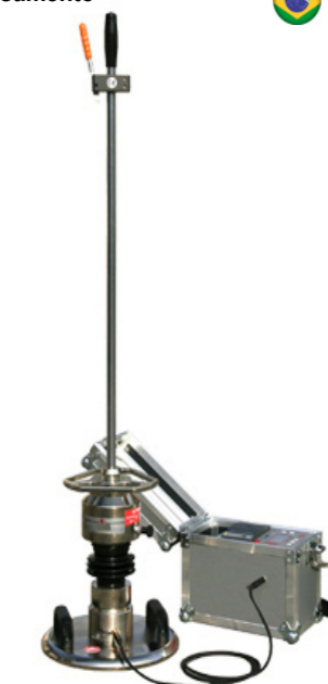
4.100.300 - LWD "Light Wheight Deflectometer"
