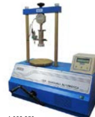
1.022.250 - Prensa CBR / Marshall Digital Microprocessada
